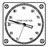
Look at the gauge attached to the tank with numbers from 5 to 95. Numbers indicate the percentage of gas remaining in the tank. If your tank gauge reads 25% or less, call your propane supplier for a refill. We recommend that you learn how to read your tank gauge, and develop the habit of checking it on a regular basis, especially if you choose not to participate in our company's **Keep-Full** program.
